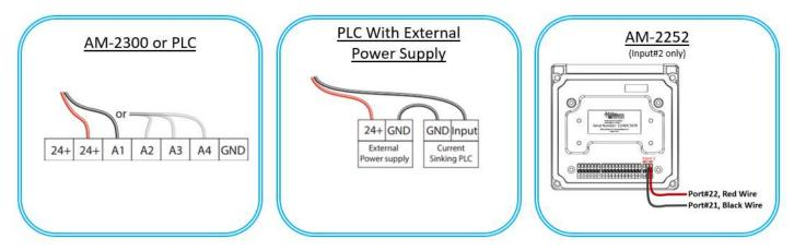
Note: the 4-20mA mapping is defaulted to 0-400mS/cm. For custom ranges, use the Digital communication protocol or contact the Water Analytics Team.
