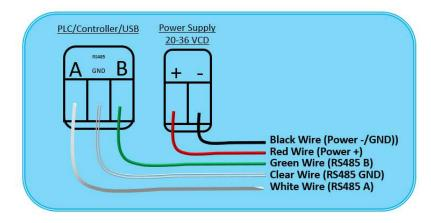
Note: Digital communication is currently available over RS485 and via CLI commands. The Modbus RTU protocol will be available in future releases.
