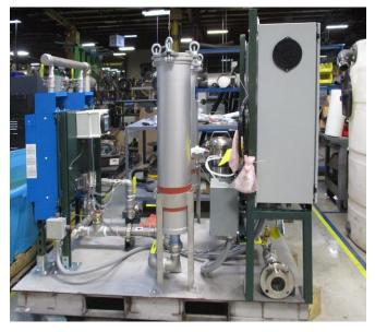
For the Watts rainwater harvesting system, pH, chlorine and conductivity sensors are connected to one AM-2300 web-enabled controller and ensure that water purity and chorine residual are within tight tolerances.
